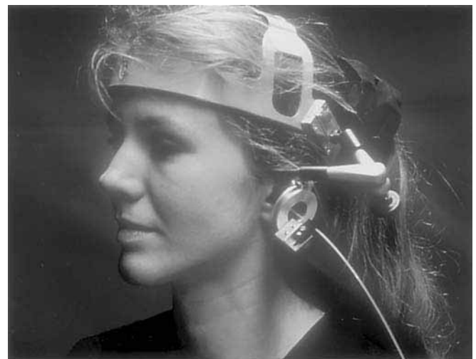
Fig. 2 The new-developed head-set applicator for the TCL-system. A synthetic headband-construction is adjusted and fastened to the upper head of the patient. The microlens laser fibre is positioned within the external auditory meatus nearby the tympanic membrane (in defined position) and is immobilised by a micro-tripod with ear speculum at the lateral site
